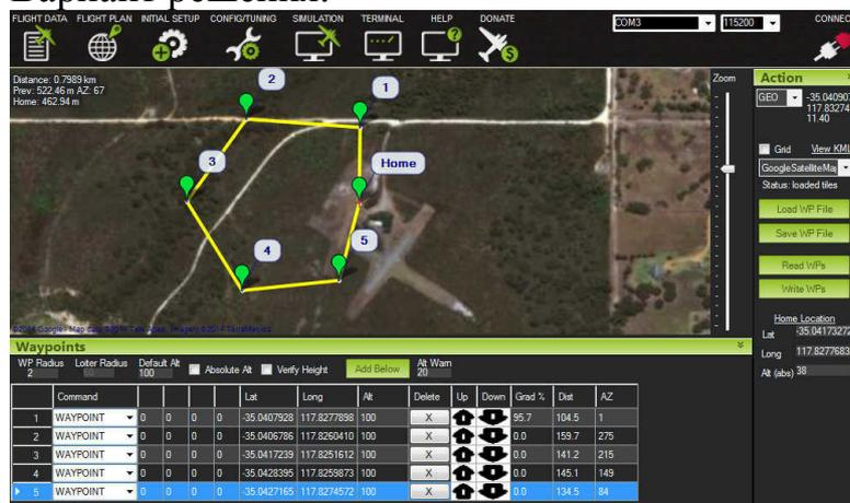
The screenshot shows the Mission Planner interface. At the top, there are tabs for FLIGHT DATA, FLIGHT PLAN, INITIAL SETUP, CONFIG/TUNING, SIMULATION, TERMINAL, HELP, and DONATE. The main display area shows a satellite map with a yellow flight path consisting of 5 waypoints, numbered 1 through 5. Waypoint 1 is labeled 'Home'. Below the map is a 'Waypoints' table with columns for WP, Radius, Lat, Long, Alt, Delete, Up, Down, Grad %, Dist, and AZ. The table contains 5 rows of waypoint data.
