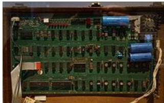
Here you can see the original 1976 Apple I Computer PCB from the Sydney Powerhouse Museum collection.
