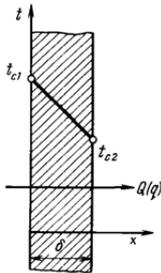
$$q = -\lambda \frac{t_{cm2} - t_{cm1}}{\delta} = \frac{\lambda}{\delta} \Delta t = \frac{\Delta t}{R}.$$
